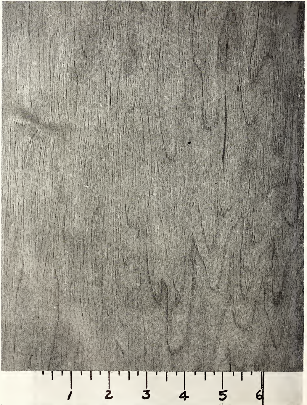
FIGURE 2-86.—Objectionable rough cutting in maple.
